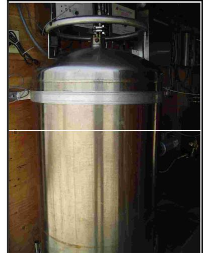
The ozone pulse-tank allows delivery of a large volume of concentrated ozone into the subsurface.
